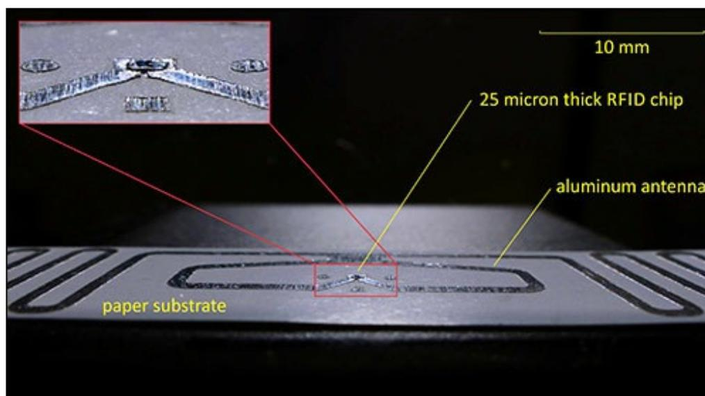
An RFID inlay made with Uniqarta's prototype first-generation process and a Walki aluminum antenna.
